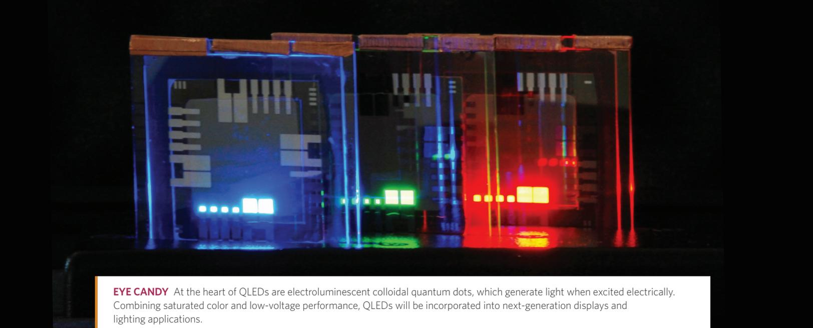
**EYE CANDY** At the heart of QLEDs are electroluminescent colloidal quantum dots, which generate light when excited electrically. Combining saturated color and low-voltage performance, QLEDs will be incorporated into next-generation displays and lighting applications.
